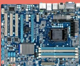
2. Three types of motherboard can be fitted to this tower (standard-ATX, micro-ATX and mini-ITX). Every other component installed in the tower is plugged into the motherboard.
