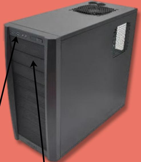
9. Two built in USB ports are installed at the front. The expansion slots could be used to add more at the back.
