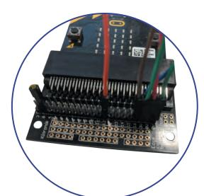
In this image you can see how the micro:bit breakout edge connector is used to connect the header cables to the relay and the moisture sensor.
