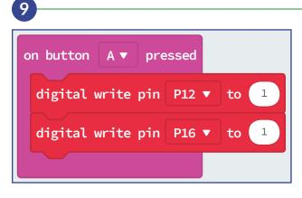
These blocks add the ability to turn off the relay by pressing the A button.
