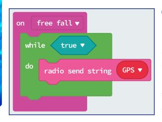
In this example, the micro:bit waits until it senses a 'free fall'. This would happen if the tree was chopped down and it fell (assuming the micro:bit is high enough up the tree!). You will need to test this!
