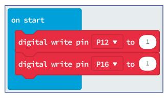
These blocks set the digital write to 1. This may seem odd as usually 1 = on and 0 = off but the relaybeing used is 'active low' which means it turns the switch on with a 0 rather than a 1.
