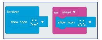
A simple interaction to start with is the micro:pet reacting to being shaken. Here, the micro:bit's accelerometer senses when it is being shaken using the **on shake** block. It then shows a sad face to represent the micro:pet being unhappy when it is shaken.
