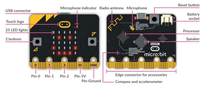
The most obvious way to tell which micro:bit version you have is by looking at the pins. The new micro:bit has notches that help keep crocodile clips attached and prevent them touching the other pins by accident when moved.
