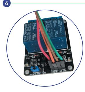
Here you can see the header wires on the relay board. Notice the cable colours and how they match the pins above.
