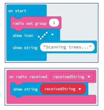
This project is designed to be created on a physical micro:bit: a node in one MakeCode project and a gateway in another project. (Second "on start" block is not needed in the MakeCode simulator.) This first block again runs as soon as the micro:bit is powered on. The 'radio group' is set to the same group as the node (this is important).
